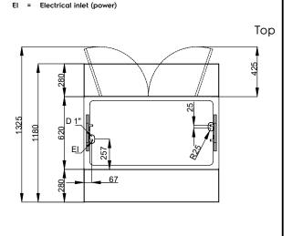
Electric Supply voltage: 220-240 V/1N ph/50/60 Hz Electrical power, max: 3.47 kW Water: Drain line size: 3/4" **Key Information:** N° of doors: 2 External dimensions, Width: 1150 mm External dimensions, Depth: 1180 mm External dimensions, Height: 1304 mm Net weight: 125.5 kg Shipping height: 1334 mm Shipping width: 899 mm Shipping depth: 1190 mm Shipping volume: 1.43 m<sup>3</sup>
